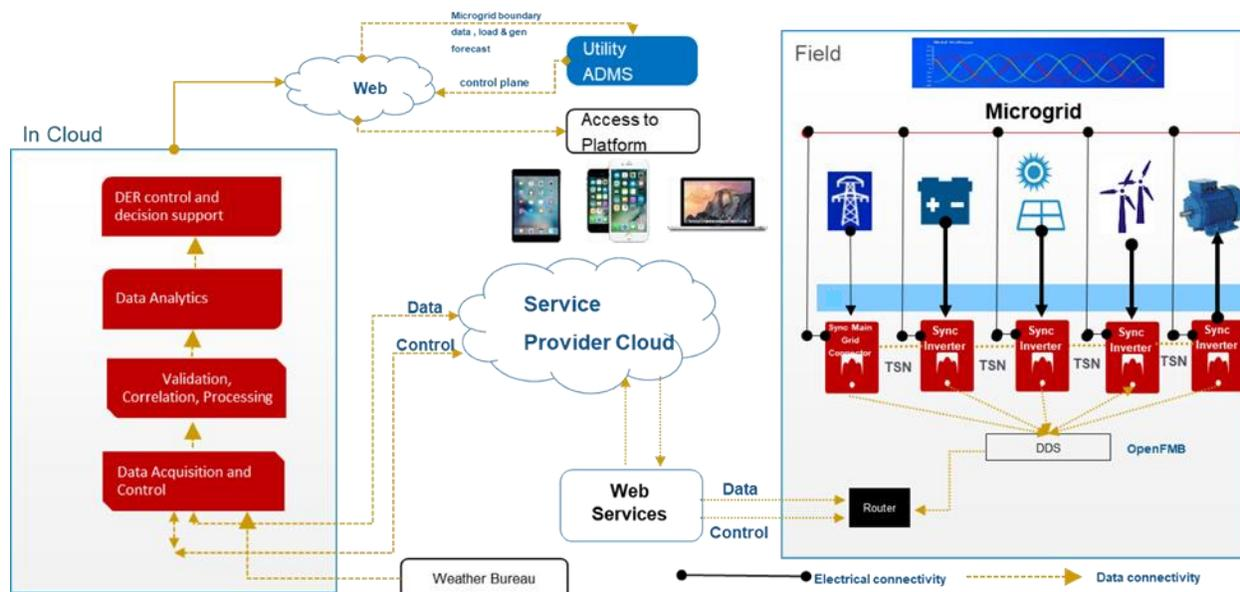
Figure 2: Deployed communication and control tiered architecture for microgrid and distribution grid management
