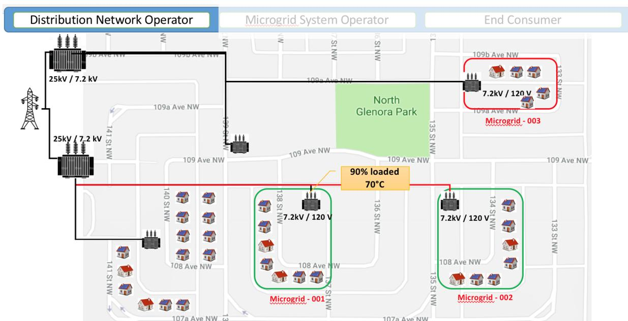
Figure 3: Distribution System Operator interface provides full visibility and control of a distribution grid with DERs and controllable loads
