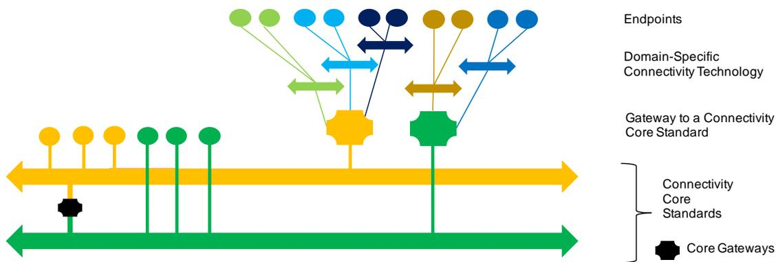
Figure 10 Standardized gateway for end-point interoperability (Source: IIC IICF)
