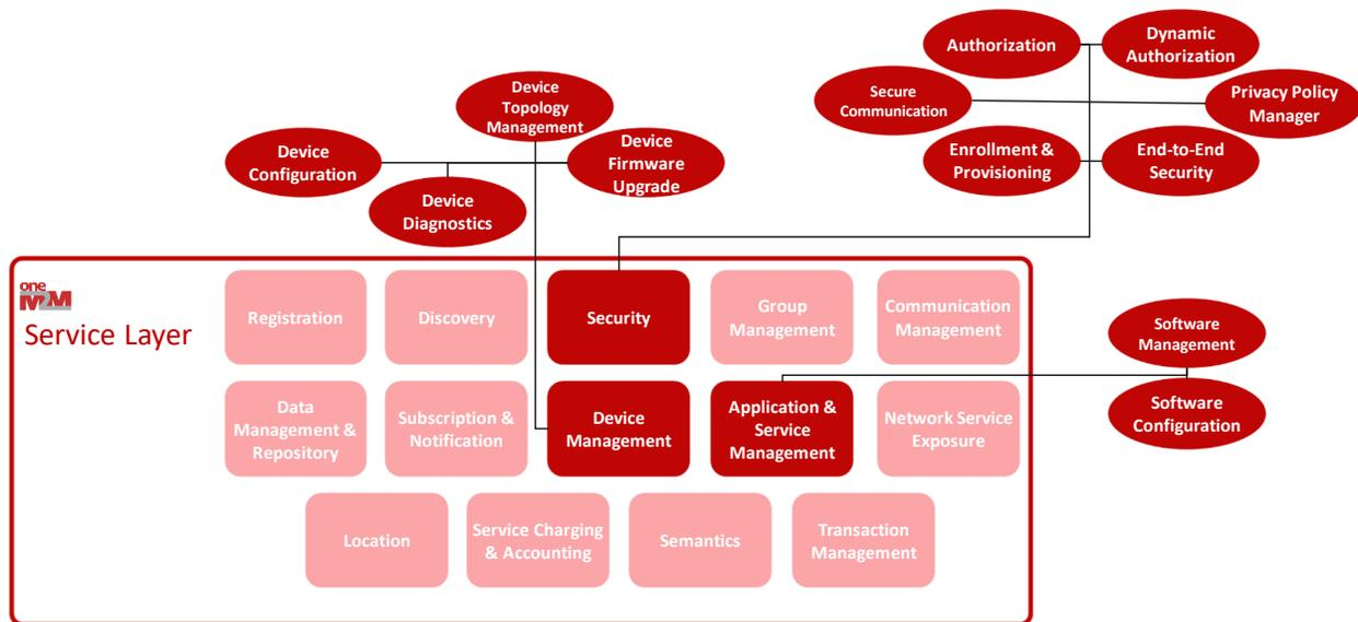
Figure 6 Illustrative Features of oneM2M Common Service Layer Functions (Source: oneM2M)
